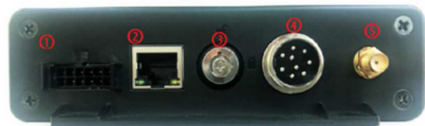
① 12PIN Socket ② RJ45 Socket ③ Lock ④ Video output socket ⑤ Wifi antenna socket
